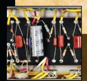
The '57 Twin-Amp gets its power from a pair of Groove Tubes®output tubes. The power supply includes Fender's rarely seen mid-'50s dual rectifier arrangement, which uses two 5U4 rectifier tubes. With this design, power amp compression or sag is
